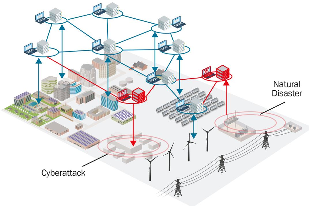
NREL is developing modeling capabilities to analyze and visualize the impacts of cyberattacks and natural hazards on the electric power system. For example, by co-simulating the grid and communications layers, researchers will better understand the interdependencies between infrastructure and find ways to optimize system architectures for resilience.
